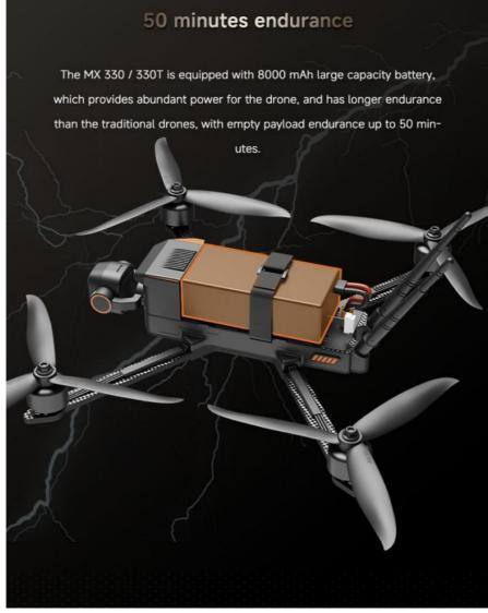
Heavy payload The MX 3301330T has super strong power,greatly improving the pay-load capacity up to 15 minutes when loading 1.5 KG.
