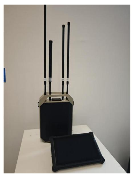
2, Device Structure and Components The DR600-A all-scenario drone detection and positioning device consists of four antenna units, a radio detection module, a video capture module, a PC terminal, a main housing, a power supply unit, and a backpack. Device Six Views:
