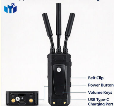
KZ-12(E) Rear Structure & Interface Design
